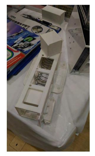
Half-size 3D print model of JEM Small Satellite Orbital Deployer (J-SSOD); BIRDS CubeSat will use the J-SSOD for its deployment from ISS
