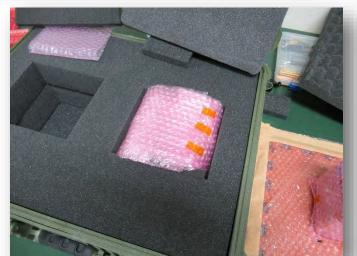
Each CubeSat was carefully wrapped with multiple layers of bubble wrap covering all sides a day before place inside Pelican box.
