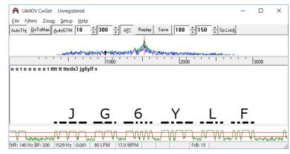
Checking CW beacon for NepaliSat-1 "JG6YLF" during Long Duration Tests
