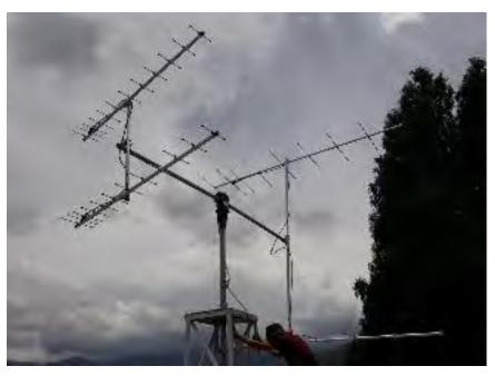
*(Up)* UHF and VHF antennas after successful installation on the stack boom
