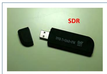
This is an SDR (software defined radio) dongle, which you can easily buy from Amazon. Most are in the \$15-\$30 range because the core component is essentially the same (a chip called **R820T/2**).
