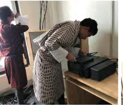
(*Up*) Mr. Rinchen and Mr. Dawa setting up the radio and connecting it with the newly installed UHF and VHF antennas.
