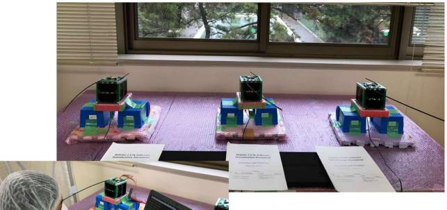
Initialization of flash memories and loading the programs to respective onboard microcontrollers
