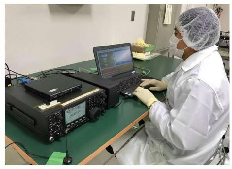
Verifying that software initialization and loading were properly done by downloading and checking the data at the ground station
