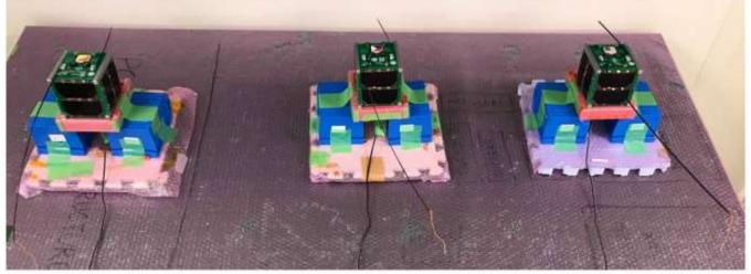
The three flight models after the successful antenna deployment test, ready for operation with the ground station.
