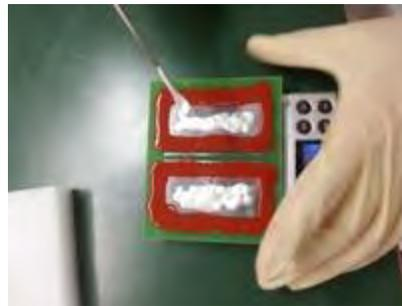
Adding RTV and Dotite to PCB
