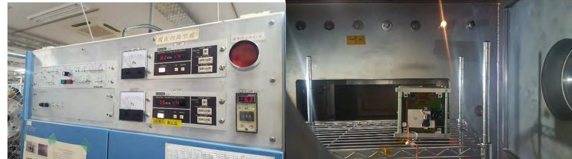
*Vacuum chamber---to check whether antenna will work under vacuum condition or not*
