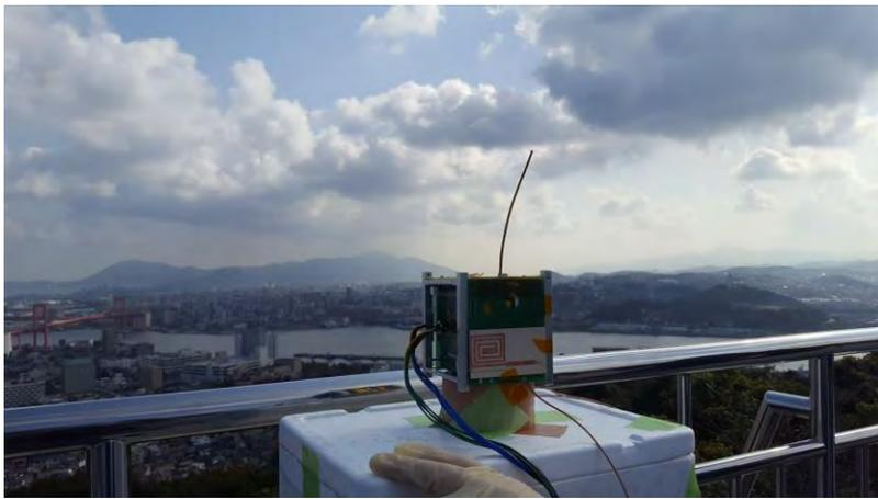
**Long Distance test-** To simulate the same distance as close to BIRDS Satellite altitude in worst case scenario (distance of 1500km) and verify BIRDS satellite uplink and downlink communication by Antennas
