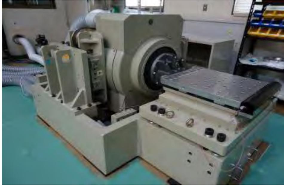
Vibration Testing Machine, Center for Nanosatellite Testing, Kyutech
