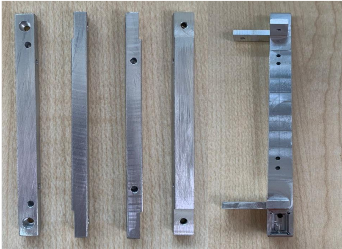
Fig. 4: Some of the parts (rails/frames) of the main structure of the ASEANSAT's CubeSat that were fabricated by SIRIM. Since the objective of fabricating the structure subsystem is to speed up the integration and configuration process of the CubeSat for testing purposes, the manufacturing of the structure was made without aluminum anodizing operation.
