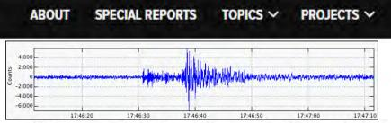
Fig. 2. Station R30E2, located in downtown Pétion-Ville, produced Haiti's first Raspberry Shake station recording of a local earthquake on 13 January 2019. This event was not reported by Haiti's national seismic network, but it was later reported by the Dominican Republic seismic network as an M3.1 event (yellow star in Figure 1) along the Enriquillo—Presqu'île du Sud fault close to the border between Haiti and the Dominican Republic.
