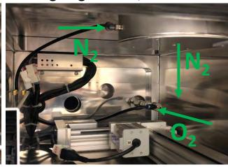
IC feedthrough for sample collection
