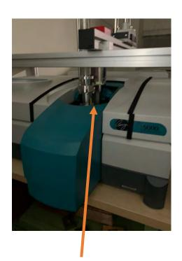
Insertion of the VTV inside the measurement zone
