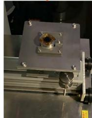
Attaching the sample holder to the sample stage in the EB machine
