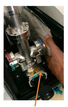
Adjustment of the VTV inside the spectrophotometer
