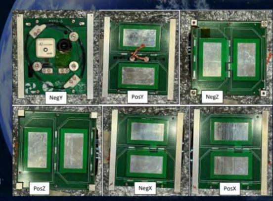
Left: Torque markings on Maya-6 EM's external panels and rail deployment switch screws before VT. Right: Torque markings on Maya-6 EM's external panels and rail deployment switch screws after VT.
