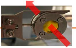
Optical window for measuring optical properties
