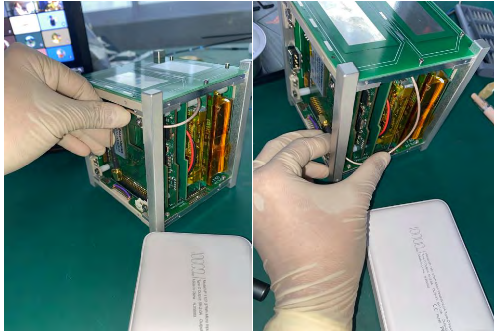
Previous (left) and new (right) configuration comparison to check for possible stress points on the SMA jack to avoid lifting
