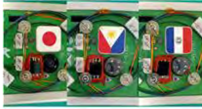
Fig 1. Perovskite solar cells attached to BIRDS-4 satellites.
