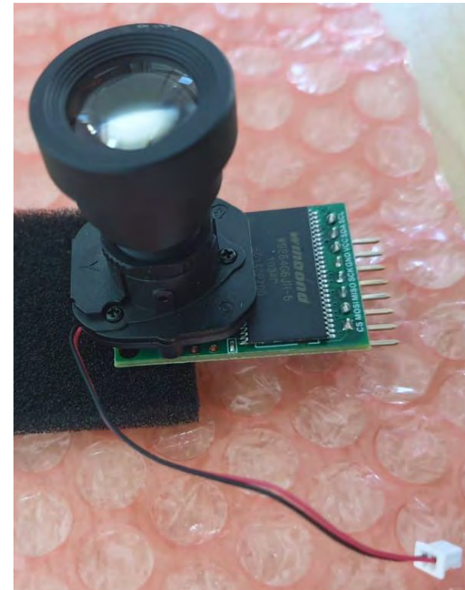
Fig. 2: The imaging sensor with 35 mm focal length lens.
