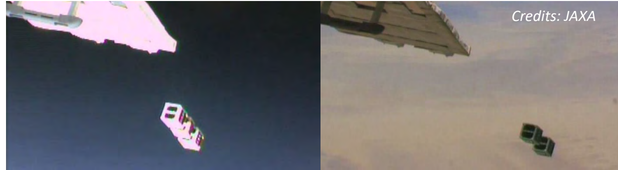
CubeSats of the BIRDS-1 are deployed from the J-SSOD. /July 7, 2017
