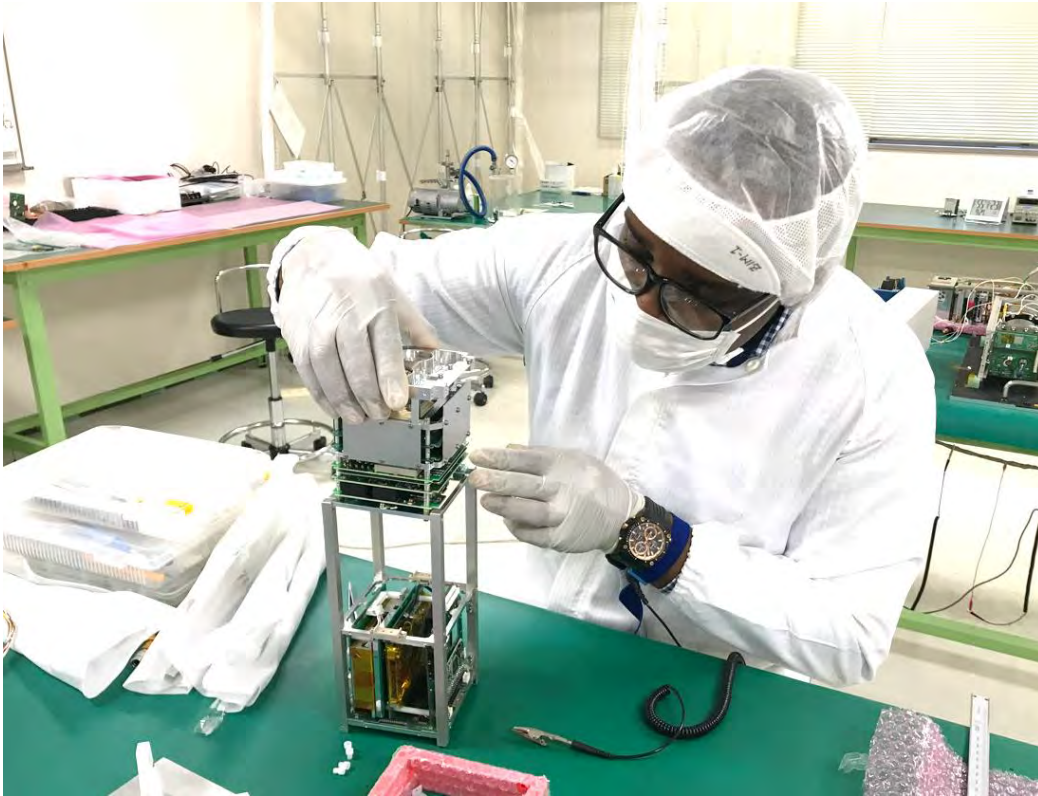
Victor trying to fit PINO module into 2U structure
