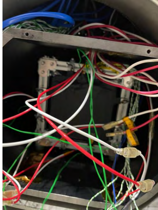
Attached thermocouples on the CubeSat inside the TVT Chamber.
