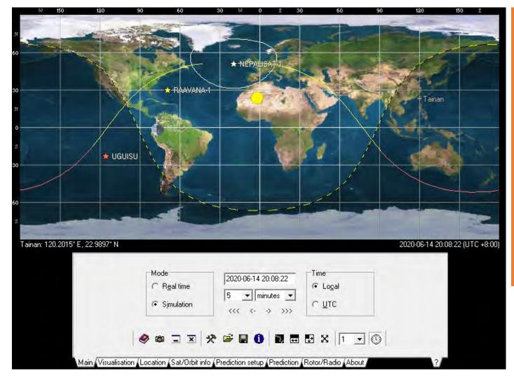
At "Main", you can change to "Simulation" mode. Set the time and step time to simulate satellite.
