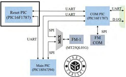
BIRDS-3 satellites have now been in orbit for a year. Radiation effects like Single Event Latch-up (SEL) can cause system to fail. The On-board Computer (OBC)'s Main PIC MCU is connected to **Reset PIC** MCU. As the name suggests, Reset PIC is responsible to listen to the "heartbeat" of Main PIC. If it stops for a designated period of time, the Reset PIC resets the Main PIC. Systems have seen to recover by resetting.
