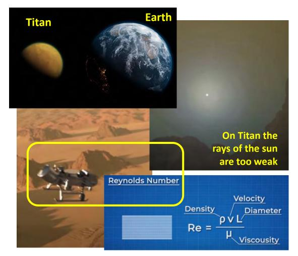
**Dragonfly** will be a rotorcraft lander, much like a large quadcopter with double rotors, an octocopter. Such redundant rotor configuration will be able to tolerate the loss of at least one rotor or motor. Each of the eight rotors will be about 1 m in diameter. The aircraft will travel at about 10 m/s or 36 km/h and climb to an altitude of up to 4 km.
