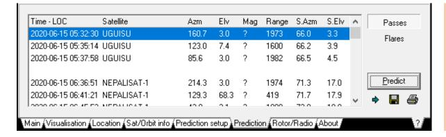
**Step5:** At "Prediction", click Predict button. You can get the time of arrival, the time at max elevation angle, time of leave and some other information based on your set up at step3. At this step, you have already finished the prediction about satellite basically.
