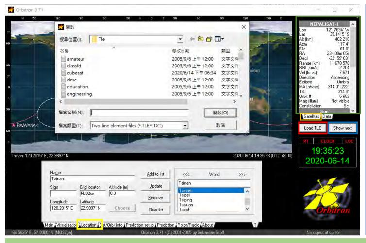
**Step1:** Open Orbitron.exe and click "Load TLE" button as shown at red box. There are different kinds of satellites you can choose. BIRDS satellites are classified into "cubesat".
