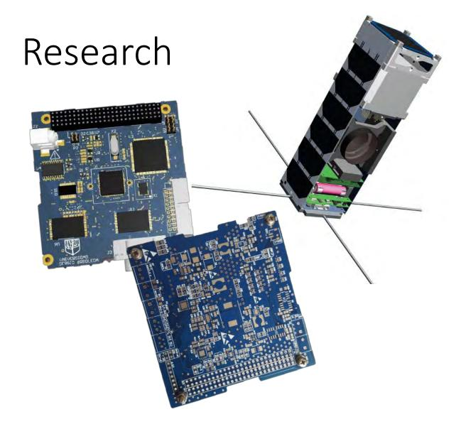
Design of subsystems for CubeSats, 3D model and manufactured PCB.
