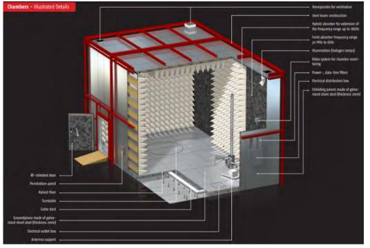
An illustration of an RF anechoic chamber [source]
