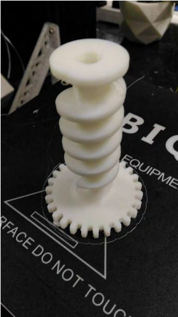
▷▷ Spur to worm gear translation
